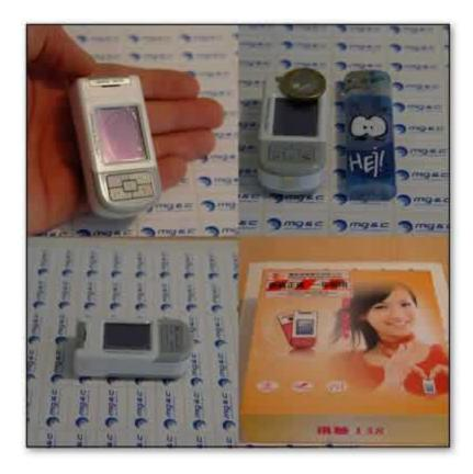
Weighing in at only 55 grams, the Xun Chi 138 is a close competitor to the Modu Mobile in terms of being lightweight. It uses a touch screen with handwriting recognition to avoid requiring a keypad, a feature that many of these small phones are starting to implement. This one's available in China where it can barely be seen in the palms of its owners because of its small size.
