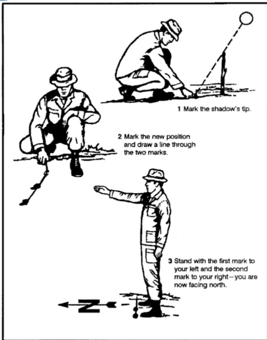
Figure 18-1. Shadow-tip method.
